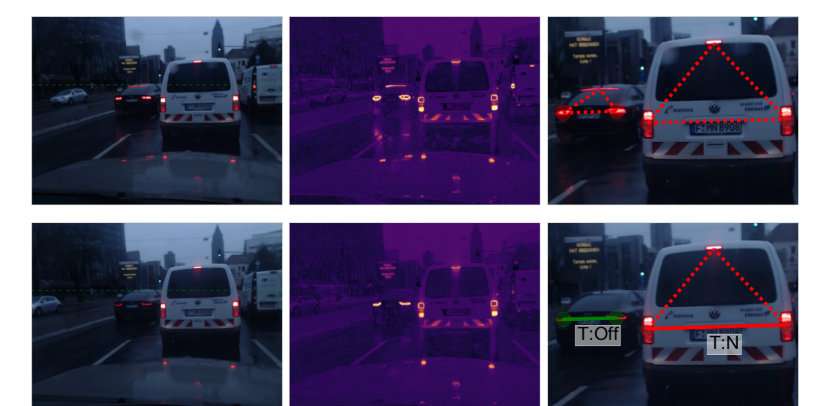
Figure: Two frames from a braking event (top: time t , bottom: t+1 ). First column: input images, second column: map of C_R , third column: magnified transition estimations (T:Off-transition from on to off, T:N-no transition detected.)
