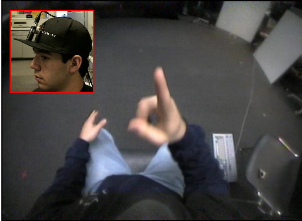
Figure 10.16 Gesture tracking from Starner et al. (1998). A camera was mounted on a baseball cap looking down at the users hands (inset). The camera image (main figure) was used to track the hands in a HMM based system that could accurately classify a 40 word lexicon and worked in real time. Each word was associated with four states in the HMM. The system was based on a compact description of the hand position and orientation within each frame. Adapted from Starner et al. (1998) ©1998 Springer.
